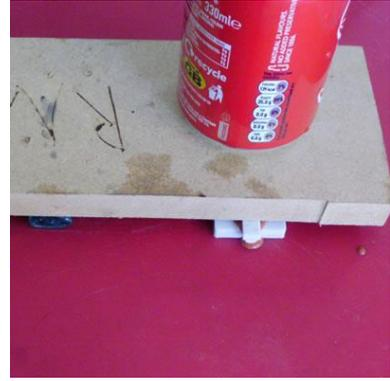
7. When the plaster has set hard remove the weight and top part of the mould.
