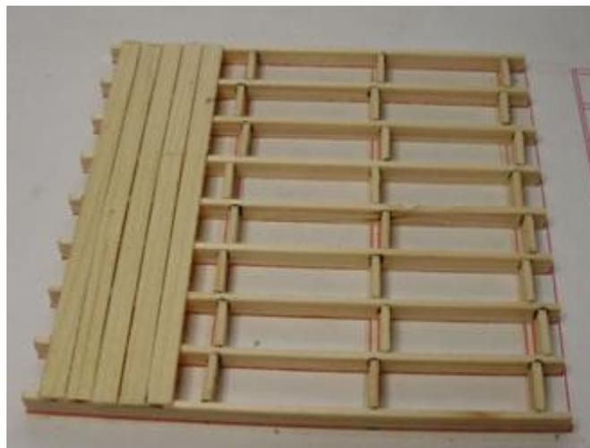
Once the floor joists have been stuck together you can stick down the floor boards. The floor boards are 0.75mm thick by 4.5mm wide.
