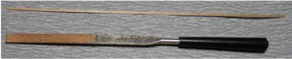
Tools we used clean and check wall section castings.
