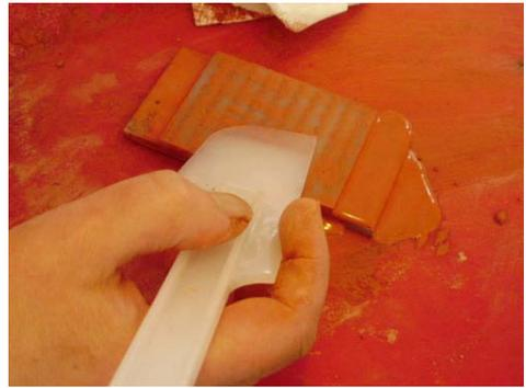
12. Let the plaster set for about 1.5 hours (terracotta casting powder) before attempting to remove the tiles from the mould. The amount of time you will have to wait will depend on the make of plaster and drying conditions.
