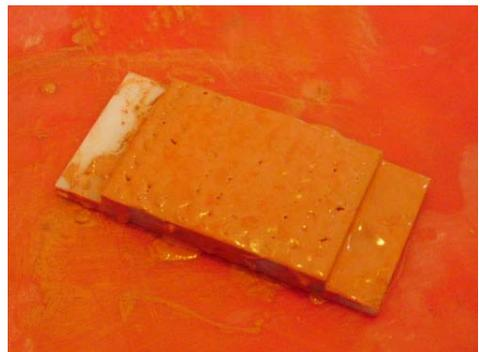
10. Cover the mould with some more plaster (if required) and vigorously tap each side of the mould until you have removed all the bubbles.
