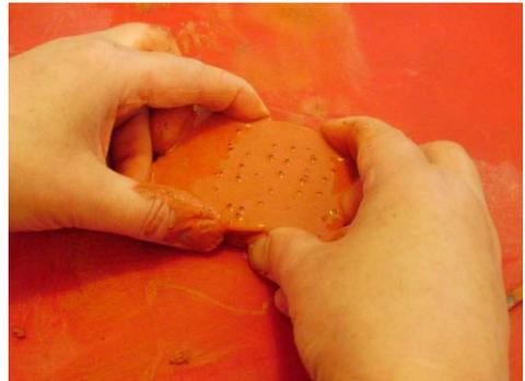
9. It is unlikely you will manage to release the mould without sucking some air back into the top part of the tile cavities.
