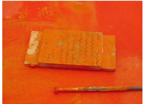
8. \*Cover the surface of the mould with 1 or 2 millimetres of plaster.
