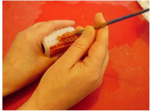
7. As mentioned before this is a messy job so clean the spilt plaster from your work surface so that the mould sits flat (*this is important because if there is any plaster under the ends of the mould they will be lift up, causing the tile cavities to close up making the tile thinner and weaker*).
